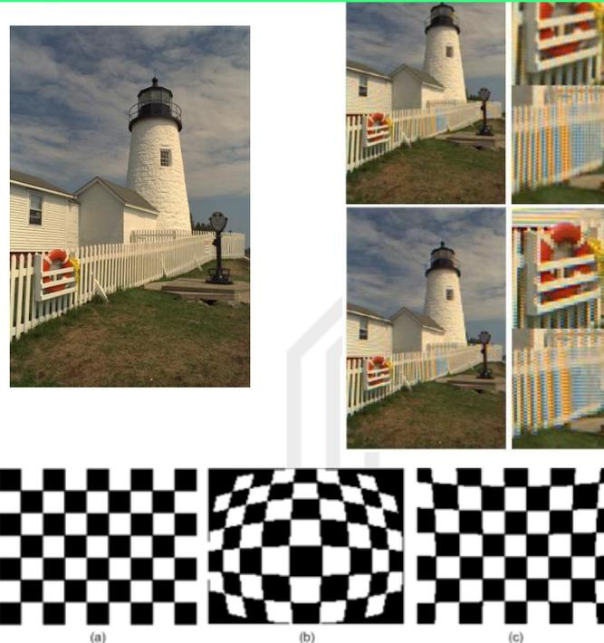
Figure 2. Examples of different types of lens distortion. (a) original (b) barrel distortion (c) pincushion distortion
